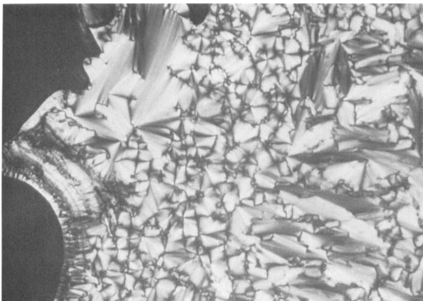
Figure 11. Contact preparation between n -nonyl gluconamide (left-hand side) and n -dodecyl-1- \beta -D-glucopyranoside (right-hand side), showing that the two materials are continuously miscible in their liquid-crystal phases.
